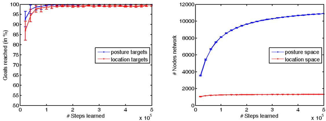
Figure 4: With even lower TGNG thresholds, the networks grow bigger and the target reaching performance also reaches close-to 100% even when reaching for location targets.
